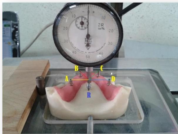
**Figure 4:** Measurements of the vertical coordinates of the abutment of implant (A, B, C and D) in relation to the reference point on the acrylic resin model (R).
