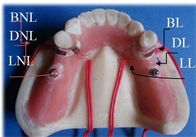
Figure 2: Strain gauges positions around premolar abutments in loading and non-loading side. BL; Buccal on loading side), LL; Lingual on loading side, DL; Distal on loading side, LNL; Lingual on non-loading side, BNL; Buccal on non-loading side, DNL; Distal on non-loading side.
